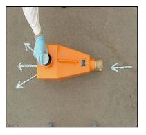
Typical Dechlorinator with De-Chlorination Tablet
